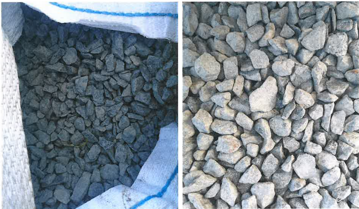
Abb. 2: Verwendete Substrate, links: Splittgemisch 8/16, rechts: Splittgemisch 16/32
